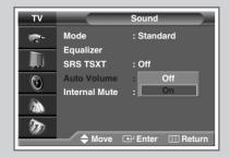
Each broadcasting station has its own signal conditions, and so it is not easy for you to adjust the volume every time the channel is changed. This feature lets you automatically adjust the volume of the desired channel by lowering the sound output when the modulation signal is high or by raising the sound output when the modulation signal is low.
